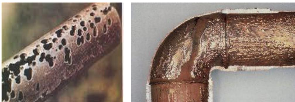
**Plate 1. The effect of corrosion on metal pipes**
