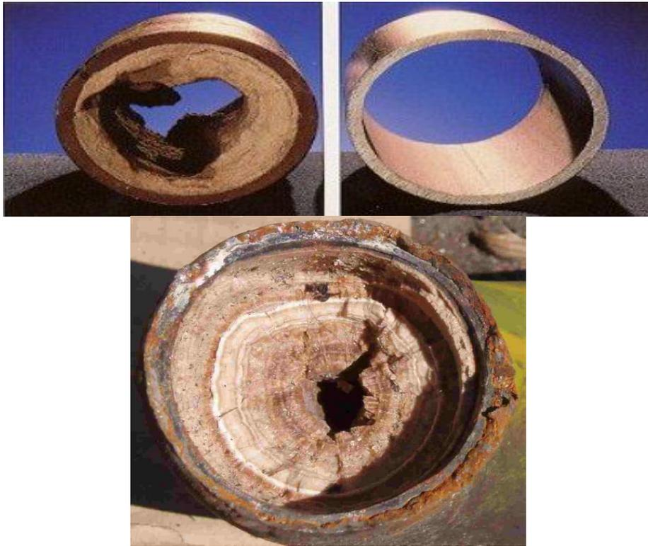
**Plate 5. Scales formed in pipes**
